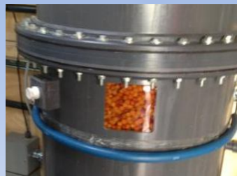
CSTR Reactor with recirculation sponges
