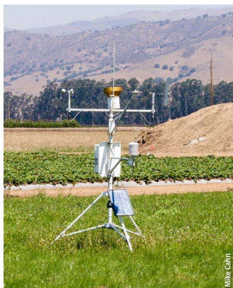
An on-site CIMIS weather station provided accurate evapotranspiration data. Each N treatment was evaluated at two levels of irrigation — 110% and 160% of ET_c .
