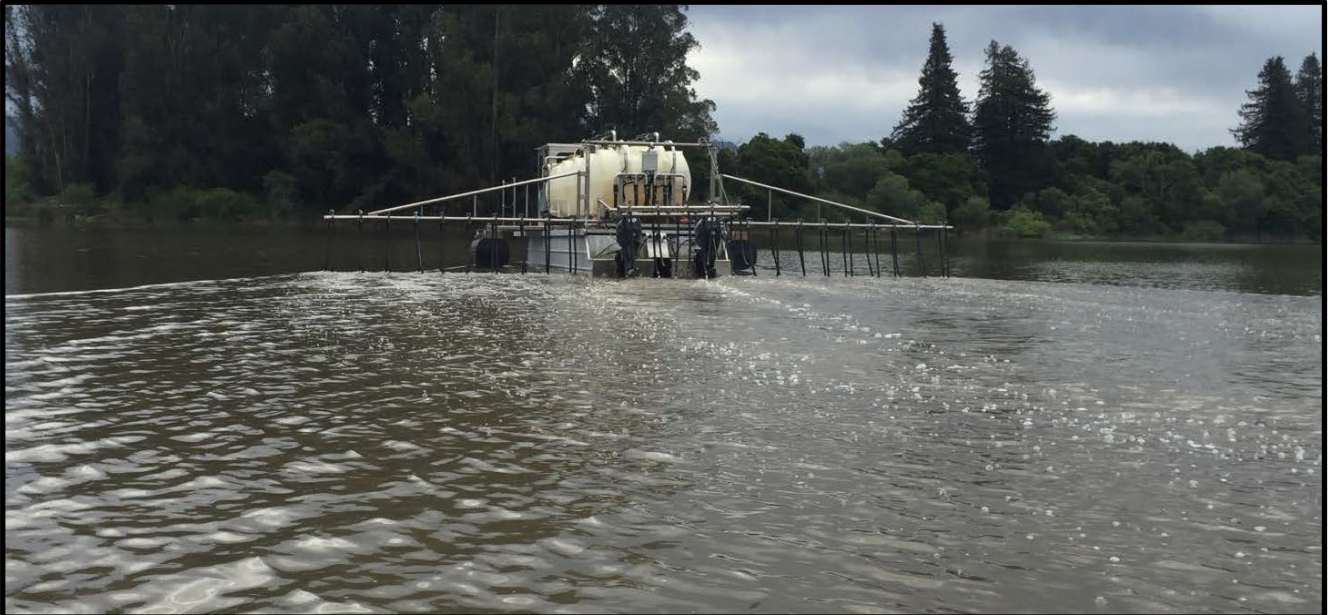
Figure 4-3. Photo: HAB Aquatics applies alum to Pinto Lake, April 6, 2017 (photo credit Catherine Bosley, HAB Aquatics).
