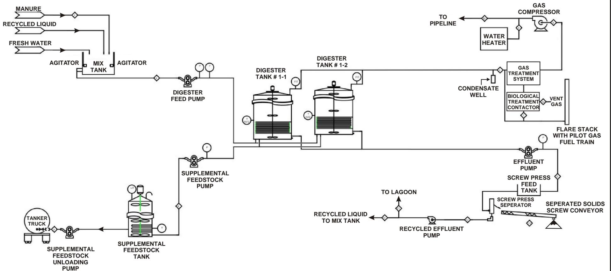
**DAIRY DIGESTER SYSTEM PROCESS FLOW DIAGRAM**
