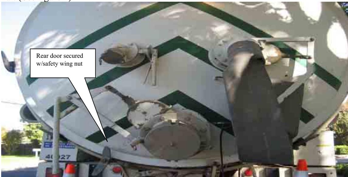
Figure 4: Rear door secured with safety wing nut installed
