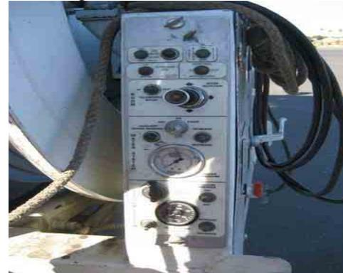
3h. Control panel for water pump & vacuum
