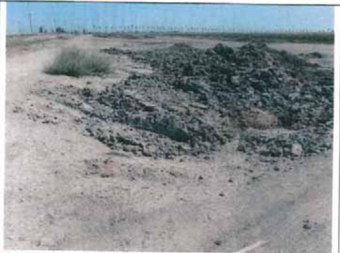
**Photo 4:** Designated manure drying / storage area. No control to convey manure leachate to wastewater lagoon.
