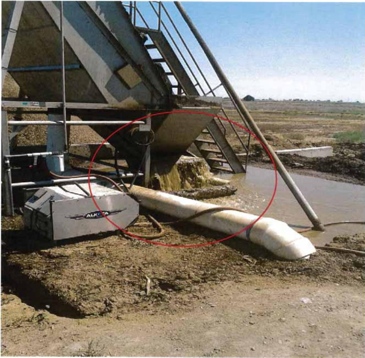
Photo 3: Photo of wastewater spilling from the broken manure solid separator during the inspection.
