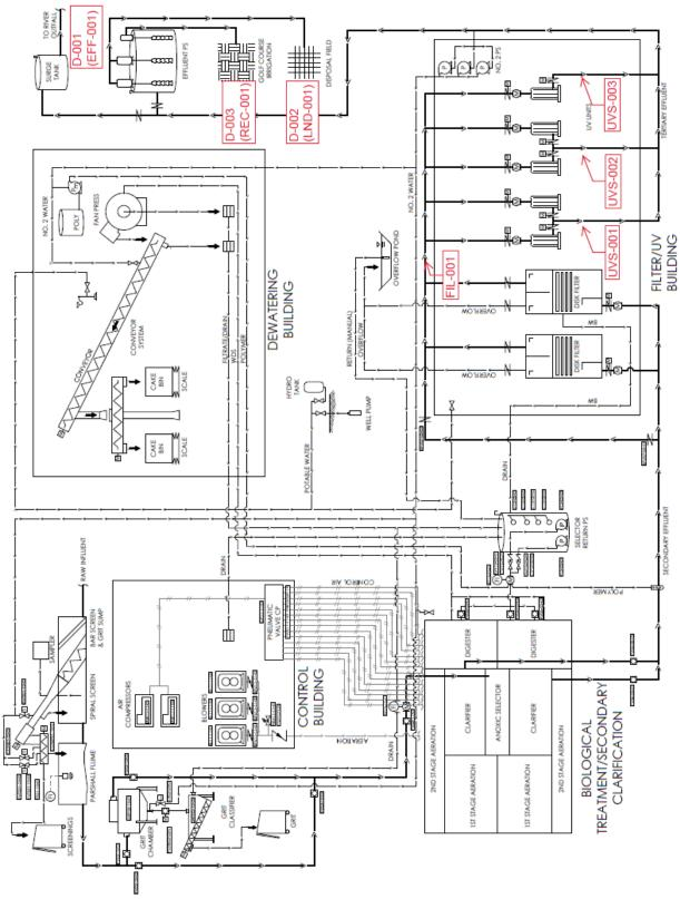
Flow Schematic for Upgraded WWTP
