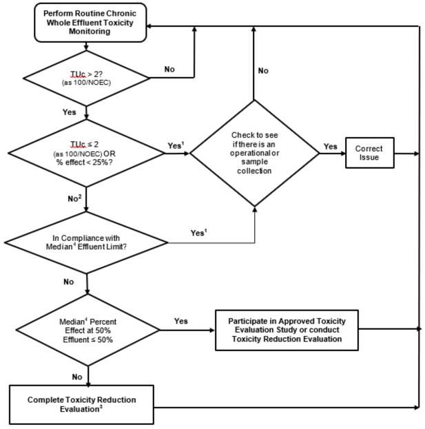
Figure F-1: WET Accelerated Monitoring Flow Chart
