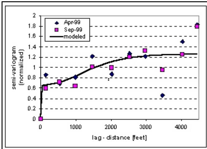
**Figure 3:** Sample semi-variograms of  $\text{NO}_3\text{-N}$  concentrations in April and September 1999. The modeled semi-variogram is a Gaussian model with a range of 1,500 m (5,000 ft), a nugget of 0.65 and a sill of 1.25 (all semi-variogram values normalized by the variance of the dataset). 1 foot = 0.3 m.
