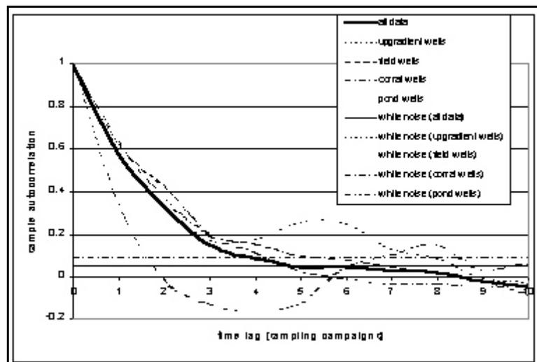
**Figure 4:** Sample autocorrelations in time for the complete dataset (solid line) and for individual management units. Estimated white noise levels are represented by the corresponding horizontal lines. Significant correlation exists only above white noise levels.
