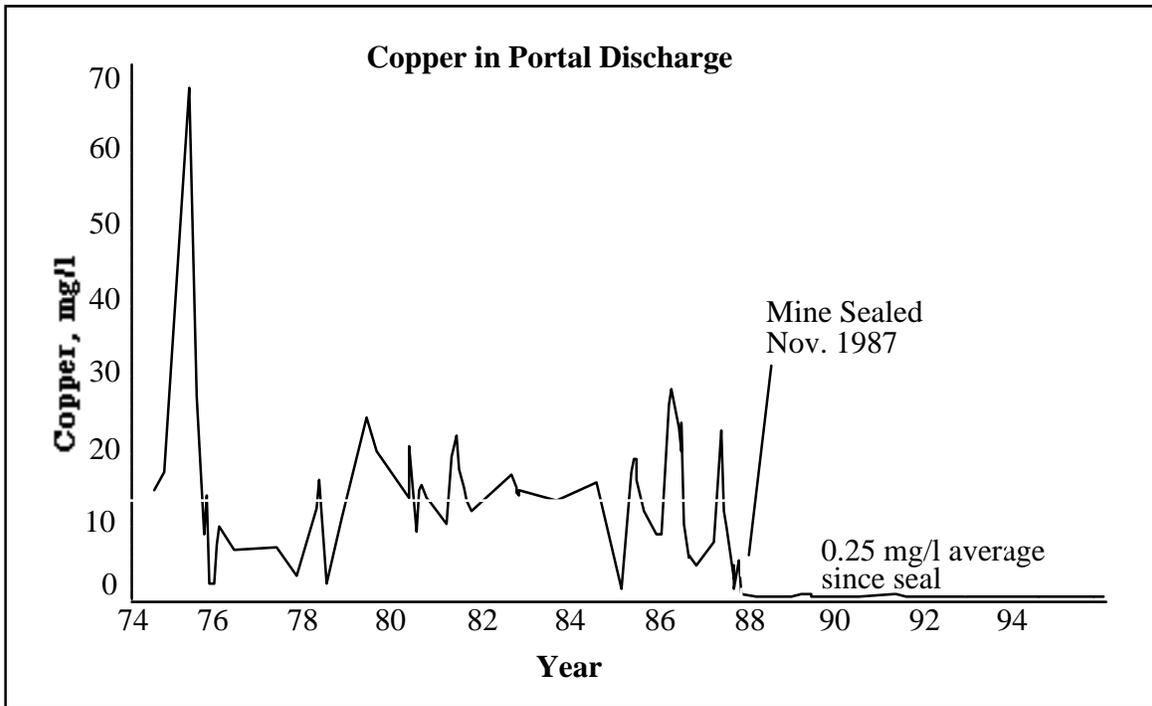
Figure 2: Walker Mine Copper Concentrations in Portal Discharge
