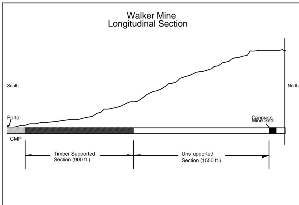
Figure 1: Walker Mine Longitudinal Section
