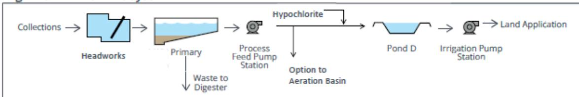
**Solids Handling Process Flow Diagram**
