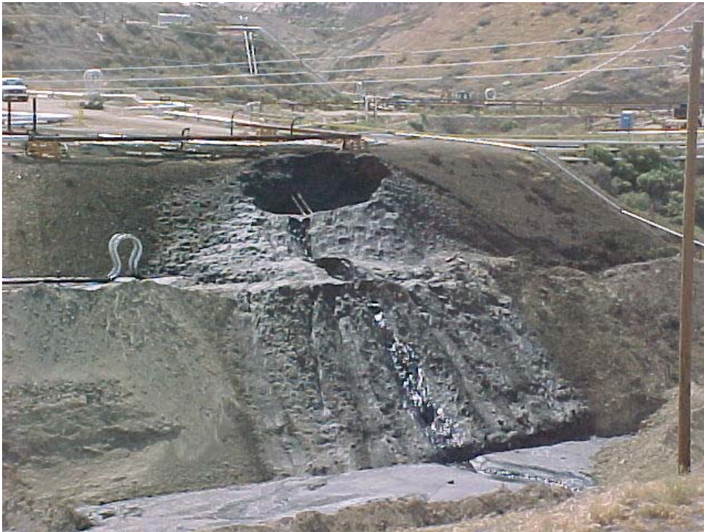
Blowout vent and debris cone. Fluid and debris within the stream channel visible in the foreground.
