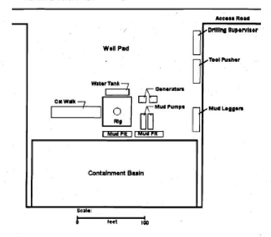
TYPICAL WELL PAD LAYOUT DIAGRAM NORTH BRAWLEY GEOTHERMAL EXPLORATION PROJECT
