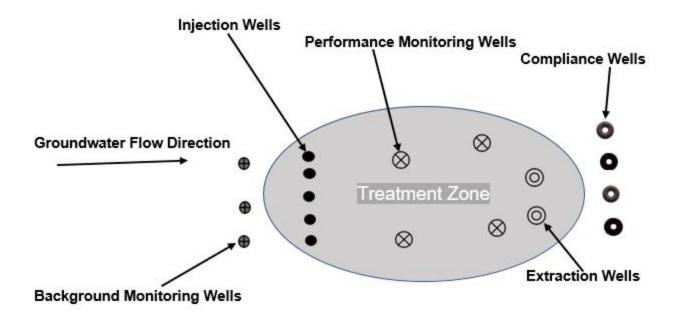
Figure 1: Generalized Monitoring Well Network Diagram
