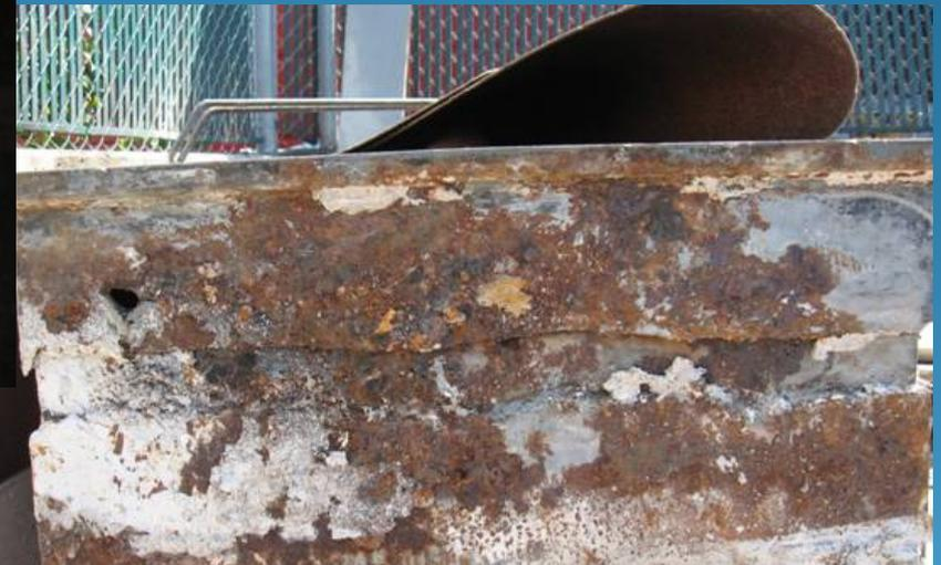
Floor trap that has rusted. Many traps that have been installed in floors were never designed for below floor installation
