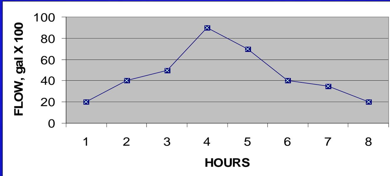
If an eight bottle discrete based sample was collected (one bottle per hour), a flow proportional sample could be prepared by using hourly flow data
