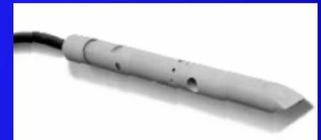
3. Bubbler - A constant flow of bubbles are continuously pushed through a small tube in the flow stream and the backpressure changes in proportion to the liquid level in the flow stream
