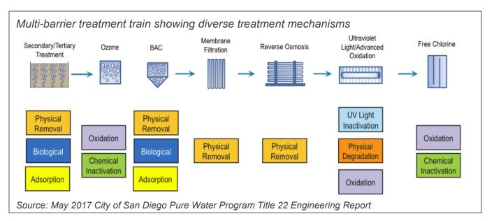
probability (*i.e.*, < 1%) of not achieving the design LRV would require considerably more sampling and is generally not practical. Requiring redundant treatment barriers is a more practical means of assuring highly consistent LRV performance. The multi-barrier concept can be enhanced for DPR by increasing the number of effective barriers required and requiring diversity of organism reduction mechanisms.
