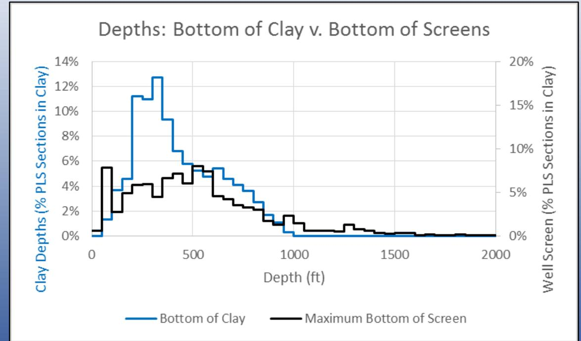
Summary of well screen depths within the extent of the Corcoran Clay from individual well completion reports. Analysis for each PLS section required to identify conduits.
