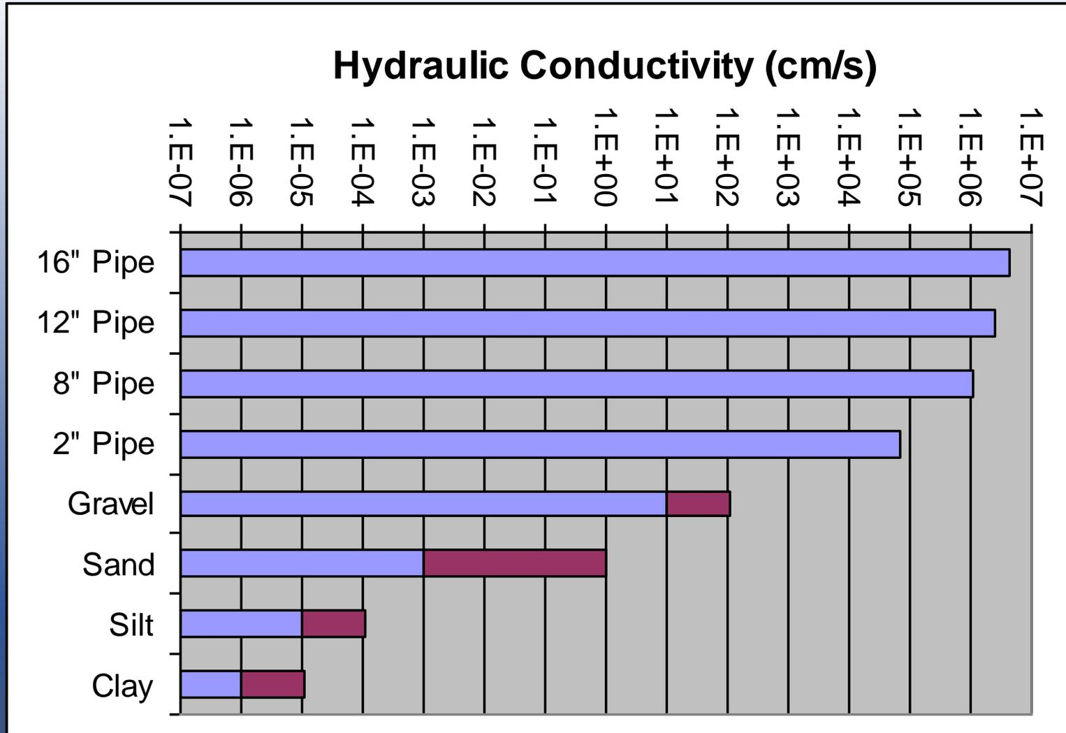
Effective hydraulic conductivities of well casings are orders of magnitude greater than layered sediments
