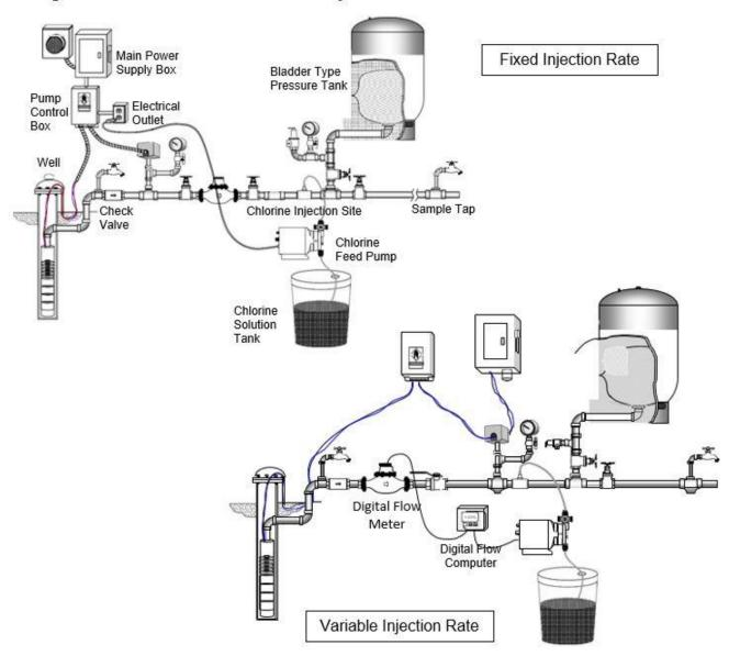
Fixed Injection Rate - If the system operates off of one well with steady flow rate, the chlorine feed pump should be electrically wired or controlled so that the feed pump activates when the well pump turns on. The chlorine feed pump injects at a fixed rate.
