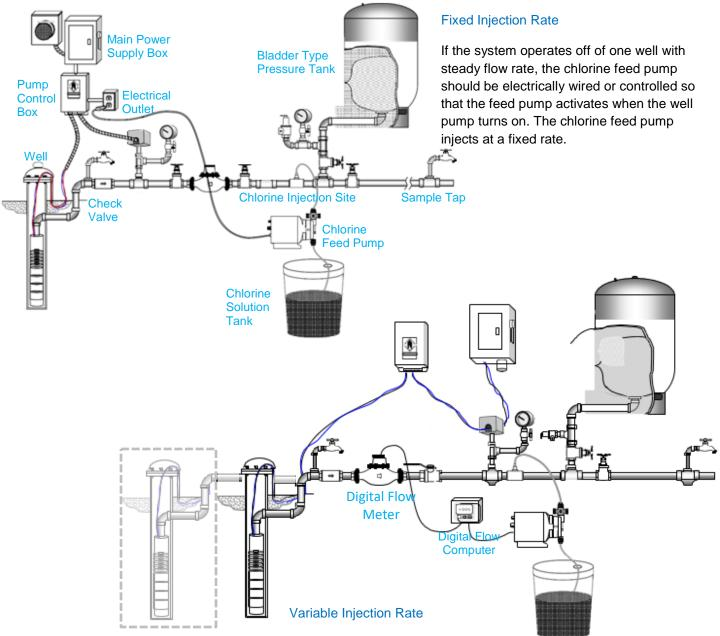
For multiple wells or if the flow of water being treated varies, the chlorine feed pump should be paced to the water flow rate. When using this type of system, the water meter sends an electrical signal to the chemical feed pump. As the meter turns faster, the speed of the pump increases, injecting the proper amount of chlorine.
