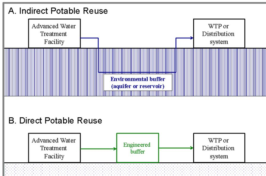
Despite the similarities between the two systems, DPR presents significant new benefits and challenges. By eliminating the environmental buffer, DPR can significantly reduce the energy
