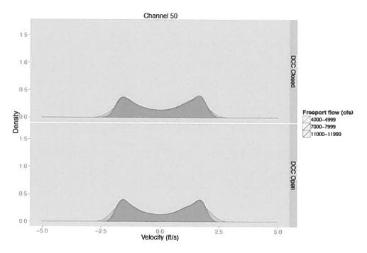
Figure 12. Density plot of velocity (ft/s) observed at DSM2 node 50 (approximately West False River) for three outflow ranges.
