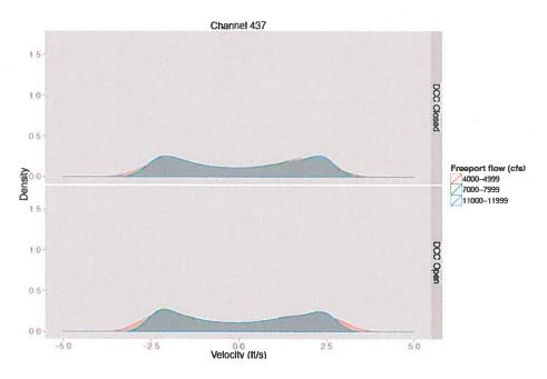
Figure 11. Density plot of velocity (ft/s) observed at DSM2 node 437 (approximately Chipps Island) for three outflow ranges.
