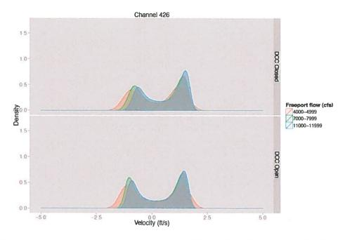
Figure 10. Density plot of velocity (ft/s) observed at DSM2 node 426 (approximately Rio Vista) for three outflow ranges.
