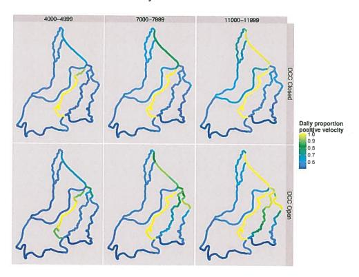
Figure 8. Maps of the North, Interior, and western Delta regions with the channels color coded for daily proportion positive velocity. Figure provided by CFS, March 12, 2014.
