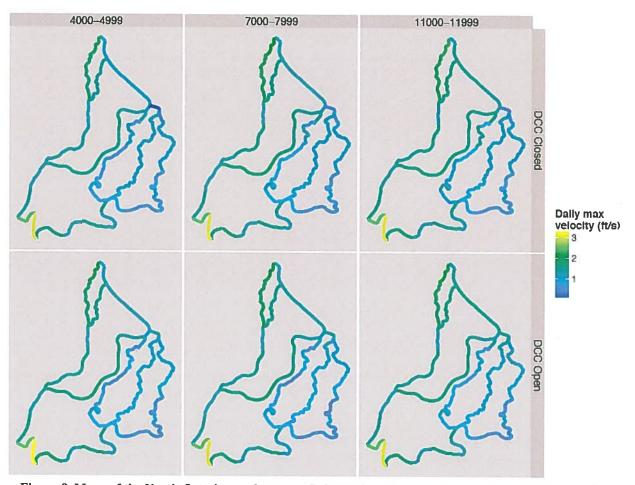
Figure 9. Maps of the North, Interior, and western Delta regions with the channels color coded for daily maximum velocity. Figure provided by CFS, March 12, 2014.
