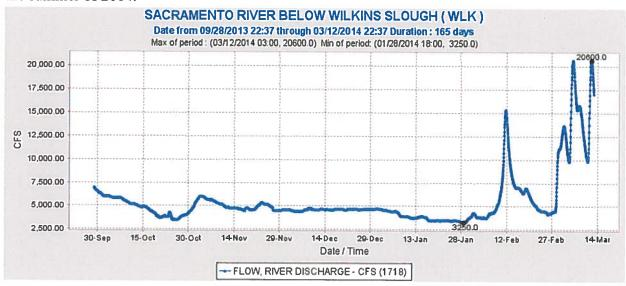
Figure 5. Sacramento River discharge (cubic feet per second) measured at Wilkins Slough during water year 2014.<sup>5</sup>
