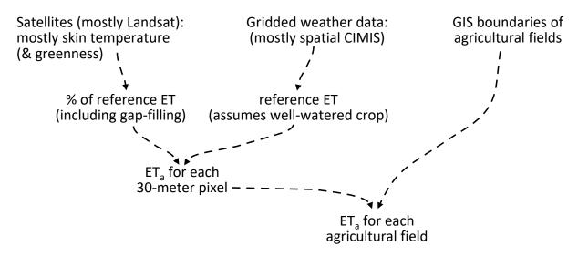
Figure 8. Simplified version of OpenET methods for calculating actual evapotranspiration (ET<sub>a</sub>). See Melton et al. (2021) for technical explanation and details.
