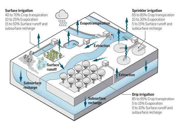
Figure 4. Diagram comparing inflows and outflows of water applied to agricultural fields through surface (i.e., flood), sprinkler, and drip irrigation. Figure cropped from Grafton et al. (2018) *Science* article *The Paradox of Irrigation Efficiency: Higher Efficiencies Rarely Reduce Water Consumption*. Values shown are general global ranges from Grafton et al. (2018), not specific to Scott/Shasta and will depend on crop and soil types, weather, and other factors.
