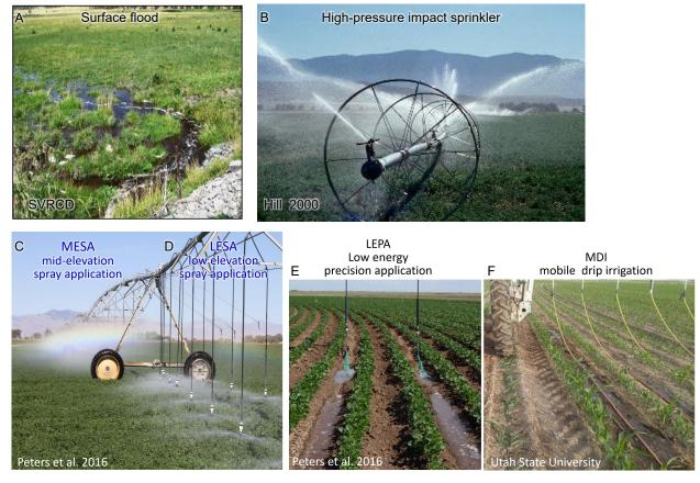
Figure 5. Photographs of irrigation technologies: (a) surface flood (b) high-pressure impact sprinkler, (c) MESA mid-elevation spray application, (d) LESA low elevation spray application, (e) LEPA low energy precision application, and (f) MDI mobile drip irrigation. Images modified from Peters et al. (2016), Utah State University (Yost et al. 2021), Hill (2000), and SVRCD<sup>3</sup>.
