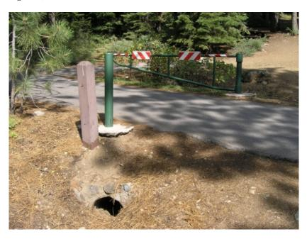
Figure 1-8. The camping spurs are very small and of variable sizes. The constrained size results in off-pavement parking and subsequent soil compaction and resource damage.
