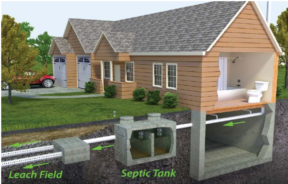
Figure 1 – Main components of a residential OWTS showing plumbing from toilets to a septic tank and to a leach field.
