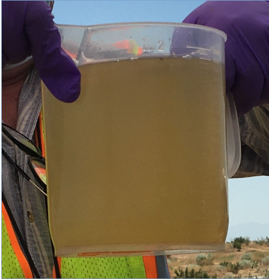
Photo 11.3 showing recovered LNAPL from a monitoring well at Site 31. Photo also illustrates the efficiency of the NET system. Traditional product recovery methods yield both groundwater and LNAPL. The measuring cup pictured above shows no detectable water during the recovery.
