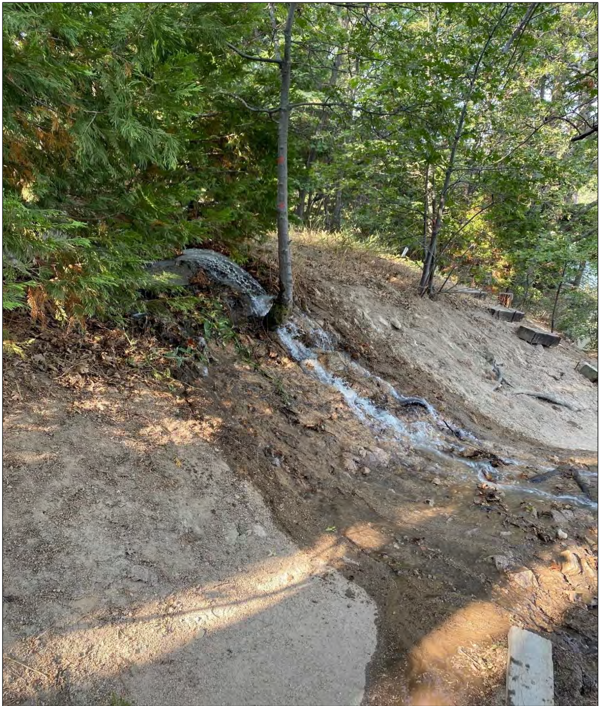
Figure 5.3 – Photograph of a July 2021, 2,900-gallon sewer line spill into Lake Arrowhead caused by blockage in the line.
