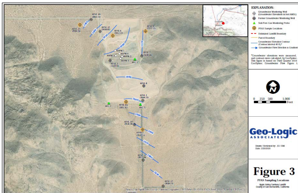
Figure 3. Map showing the Apple Valley Sanitary Landfill, groundwater monitoring well locations, and groundwater contours for the northern and southern flow regimes at this site.
