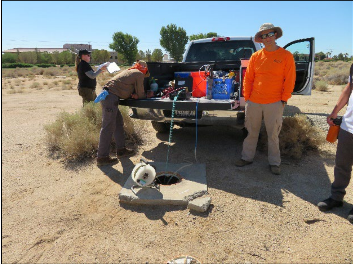
Photo 3.3: Air Force consultant field crews collecting groundwater samples using low-flow sampling methodology at Site 298.
