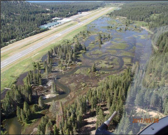
Photo 1 – Upper Truckee River Project area with over-bank river flows in late May 2017. The partially backfilled historic channel can be seen on the left side of the meadow nearest the airport runway. The newly constructed channel, which has increased sinuosity, is visible in the middle of the meadow. The goal of the project is to reconnect the river with its floodplain, which is evident in this photo showing much of the meadow flooded.
