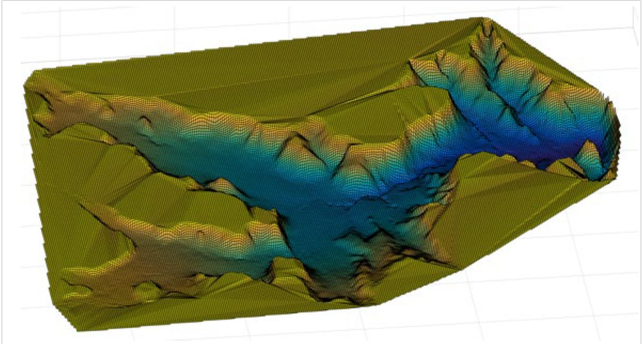
Figure 4.1 – Computer model of Lake Arrowhead bathymetry showing subsurface lakebed elevation contours. This was a necessary step to establish the computer model domain.
