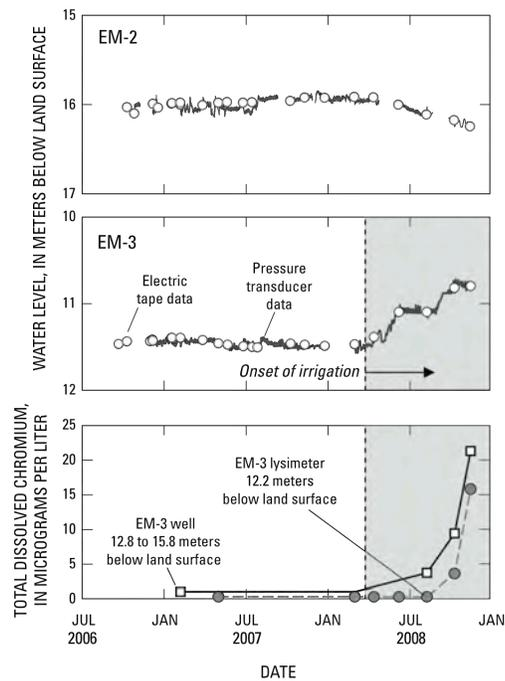
**Figure 3.**—Water-level hydrographs and chromium data for water-table wells at EM-2 and EM-3 monitoring sites, near El Mirage, Calif.
