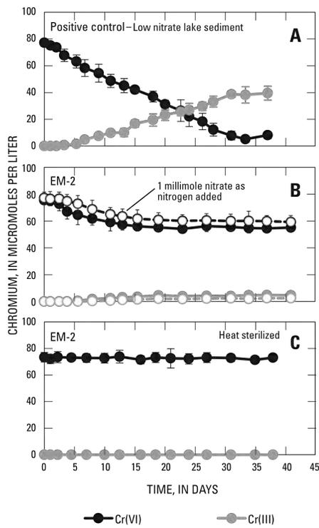
**Figure 8.**—Cr (VI) reduction to Cr (III) in laboratory microcosm experiments
