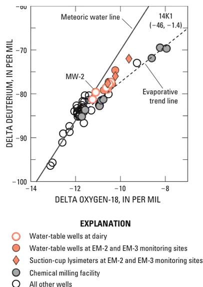
**Figure 6.**—delta Deuterium and delta Oxygen-18 composition of water from selected wells and suction-cup lysimeters near El Mirage, Calif., October, 2006 to November, 2008 (Modified from Izbicki and others, 2008a)
