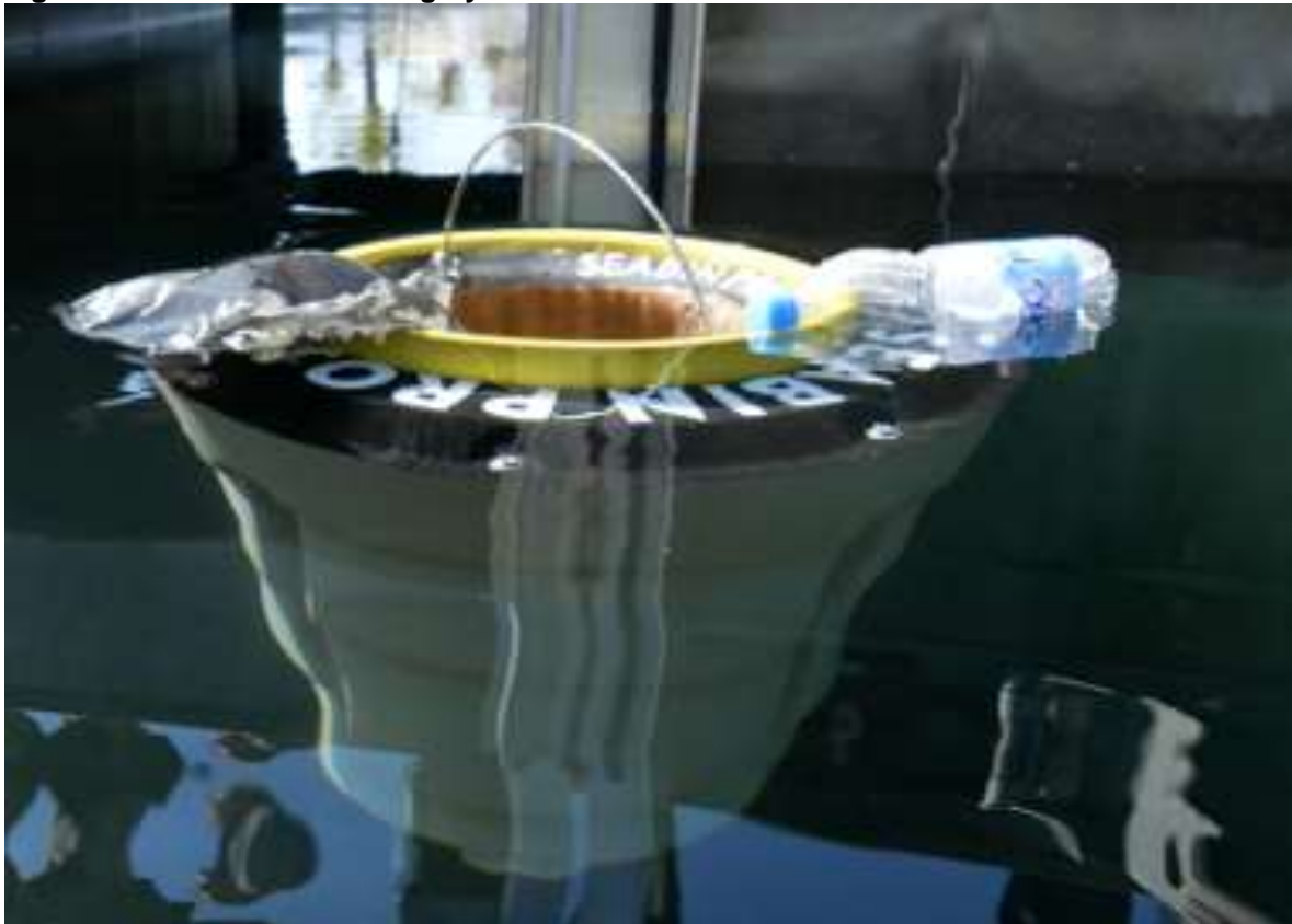
Figure 5. The Seabin Skimming System
