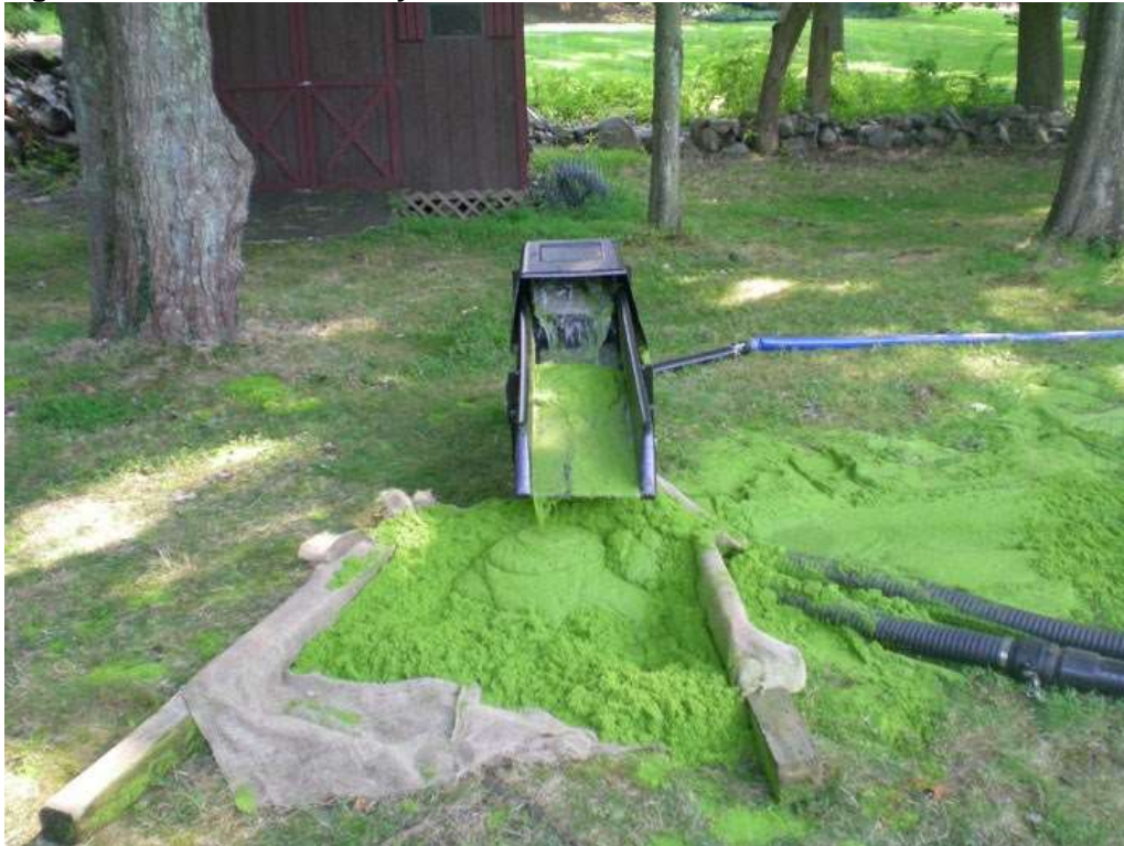
Figure 7. The ProSkimmer System – Onshore Filtration Unit
