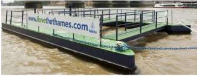
Figure 8. Passive Debris Collector, UK
