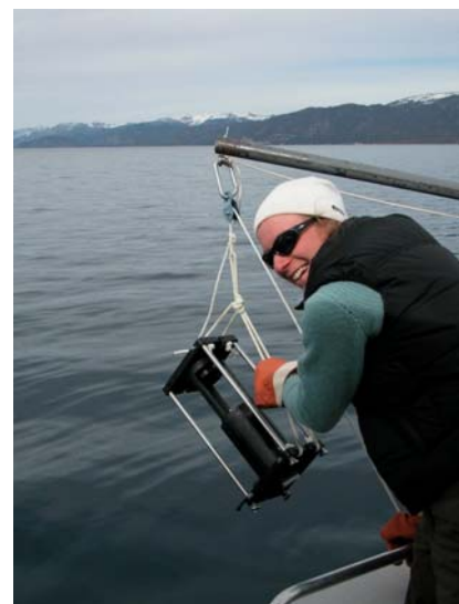
Fig. 7 Margaret Shanafield of DRI prepares an instrument used to measure how the turbidity of the water changes with depth.
