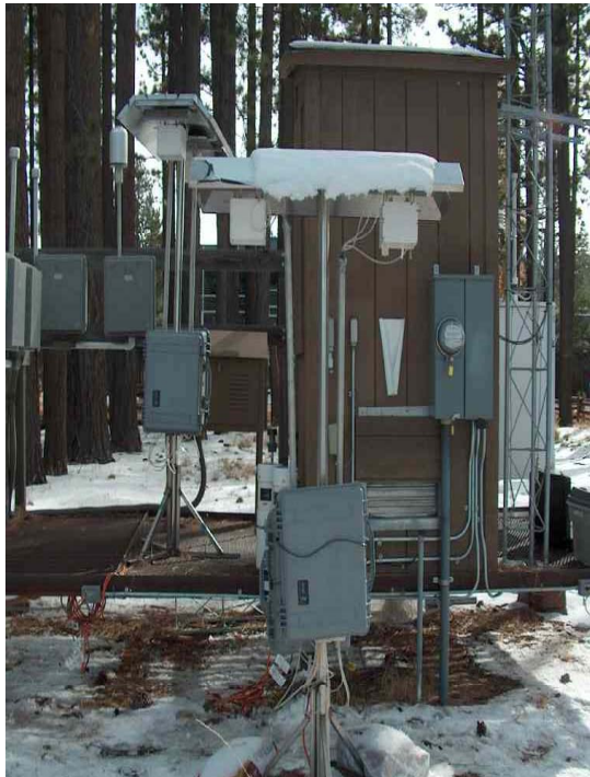
Figure 3. The Two Week Sampler (TWS) is the cornerstone of the LTADS monitoring program for nitrogen and phosphorus compounds that deposit to the Lake and contribute to algal growth. TWS measurements represent ambient conditions during every minute of the more than 1-year field study portion of LTADS.
