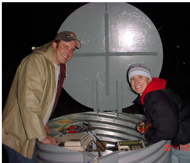
Figure 4: Raph Townsend and Andrea Parra admire a new autosampler installed in a weather- and impact-resistant housing for the TMDL stormwater monitoring project.
