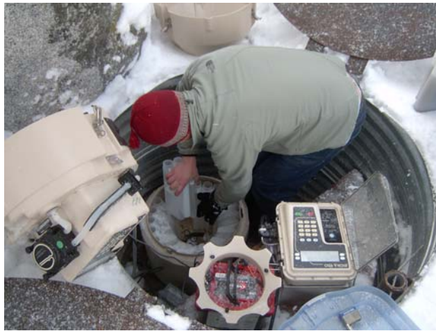
Figure 5: Shawn Beauduy collects stormwater samples collected at the South Y (SY on map below) monitoring station in March 2004. Each autosampler contains 24 sample bottles. The sampler can be programmed to collect samples of runoff on either a time interval or flow volume interval.
