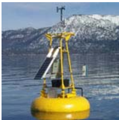
Fig. 1 NASA buoy on Lake Tahoe equipped with instruments that continually monitor the lake's temperature and surface meteorology.
