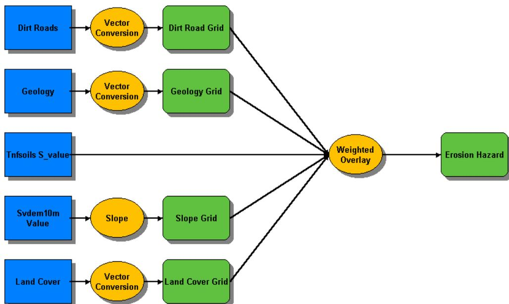
Figure 50. Flow diagram showing components of 2002 hillslope erosion susceptibility model.
