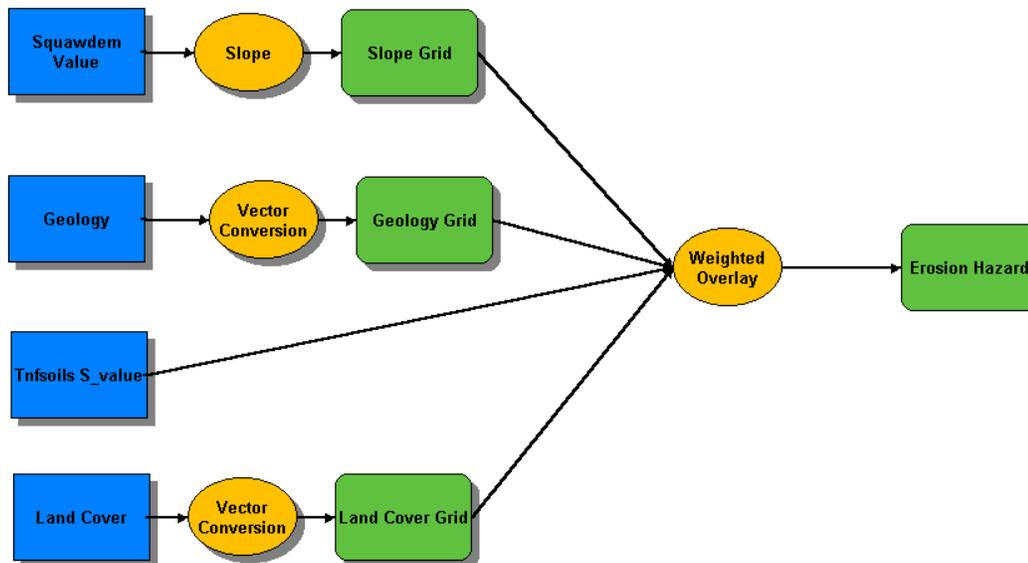
Figure 49. Flow diagram showing components of 1939 hillslope erosion susceptibility model.
