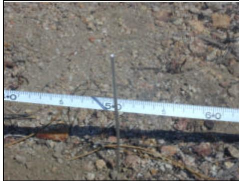
Figure 44. Erosion pin for measuring rates of sediment movement on hillslopes.
