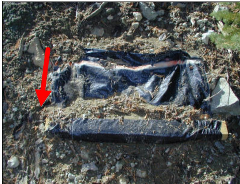
Figure 20. Erosion fence site SFII-10 below waterbar draining dirt road. Red arrow indicates downslope direction. Erosion fence is approximately 60 cm long and 9 cm high.
