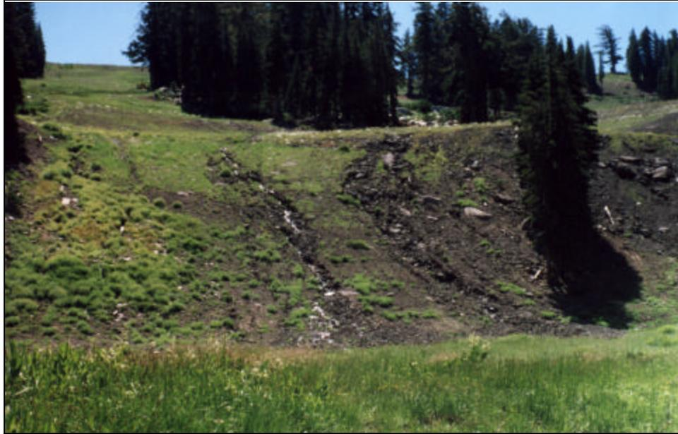
Figure 18. Rill and gully formation on graded ski run in Sector V, approximately 40 to 50 cm deep (photo courtesy of Lahontan RWQCB).
