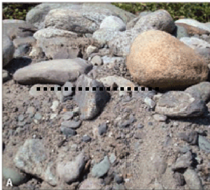
Figure 1. Typical surface versus subsurface particle size characteristics in gravel bed river substrate.
