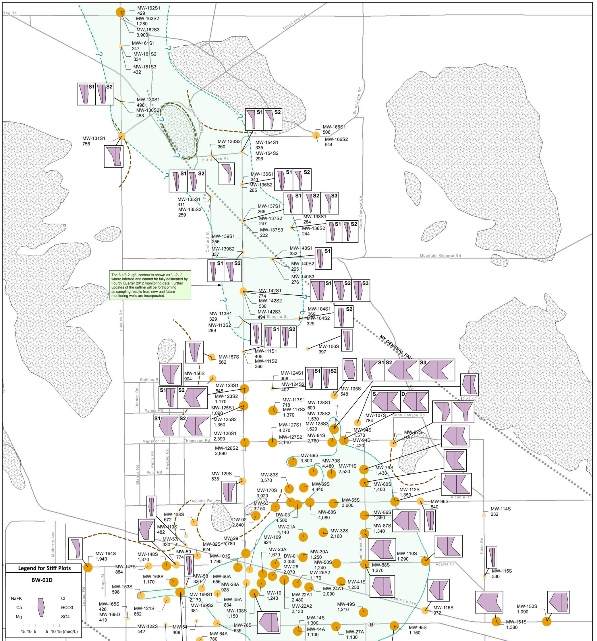
The 3.1/3.2 µg/L contour is shown as "-.-.-" where inferred and cannot be fully delineated by Fourth Quarter 2012 monitoring data. Further updates of the outline will be forthcoming as sampling results from new and future monitoring wells are incorporated.
