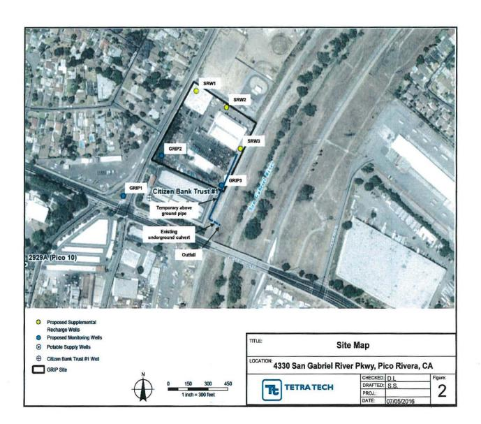
Figure 2: Injection Wells & Groundwater Discharge Locations
