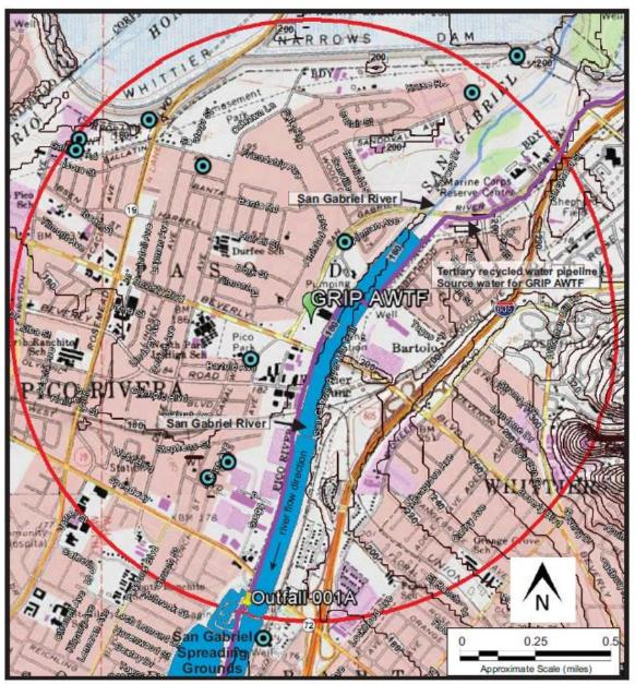
Map showing location of GRIP Advanced Water Treatment Facility (AWTF) with 1 mile radius, topography, water wells, surface water bodies, and recycled water pipeline.
