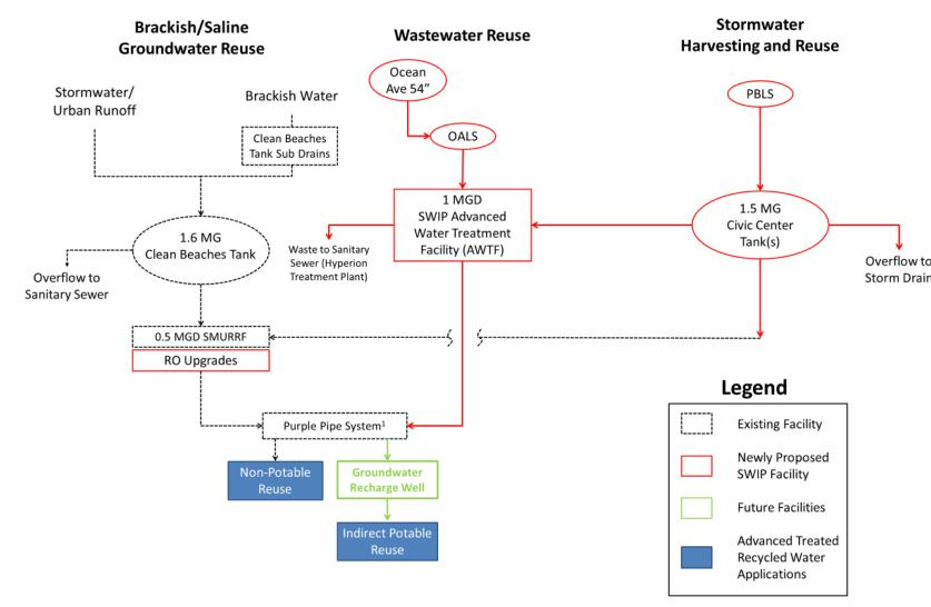
1) SMURRF and SWIP AWTF effluents are mixed within the purple pipe system connection at Ocean Ave and Moomat Ahiko Way
