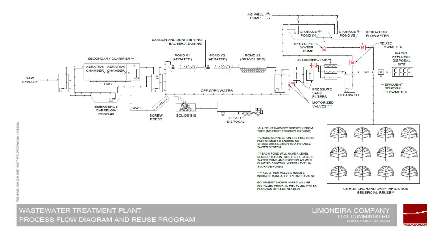
Figure 3: Process Flow Diagram
