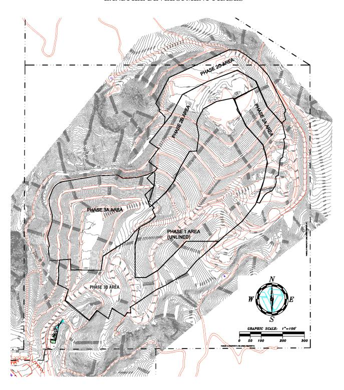
FIGURE 4: GROUNDWATER AND GAS MIGRATION MONITORING NETWORKS Abandoned Monitoring Well Gas Migration Monitoring Probe Groundwater Monitoring Well Interim Monitoring Well GRAPHIC SCALE:  $\oplus$
