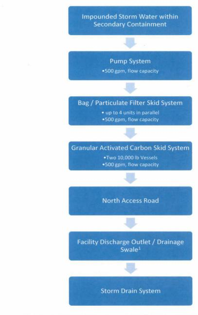
Figure 3. Storm Water Treatment and Discharge System Process Flow Diagram BP Pipelines (North America), Inc., Hathaway Tank Farm
