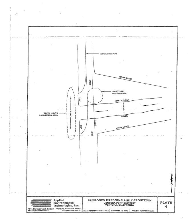
Figure 3. Zone at the mouth of the Santa Clara River for discharge of dredged material.
