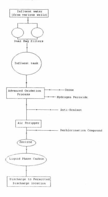
Figure 2. Treatment unit flow diagram
