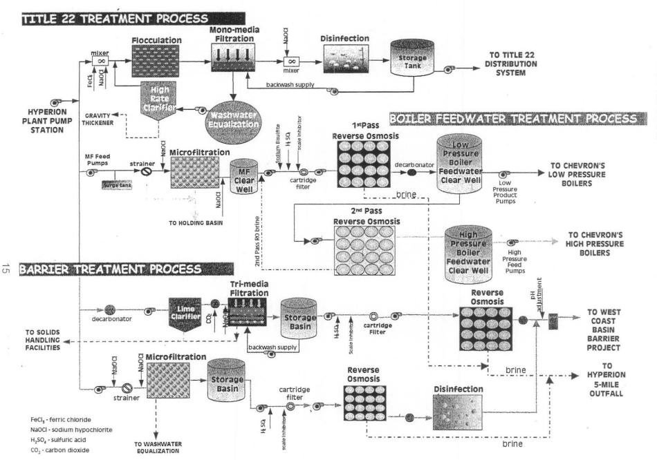
Figure 1. Schematic Presentation of West Basin Water Recycling Facility
