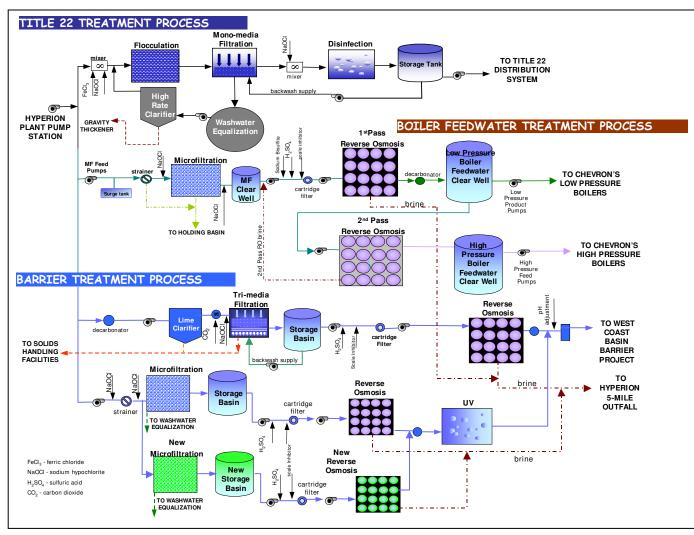
Figure P4 – Schematic of Treatment Trains at West Basin Water Recycling Plant
