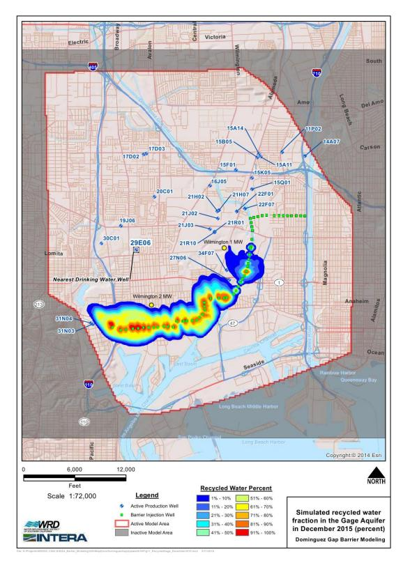
FIGURE 7 – SIMULATED RECYCLED WATER FRACTION LYNWOOD AQUIFER
